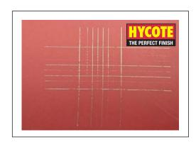
The paint film is cut in a cross pattern before pressure sensitive tape is applied. The tape is removed rapidly to assess adhesion of the paint to the substrate. The more the paint detaches from the surface of the substrate, the worse the level of adhesion. This illustrates the superior adhesion of Hycote red primer compared to leading brand A.
