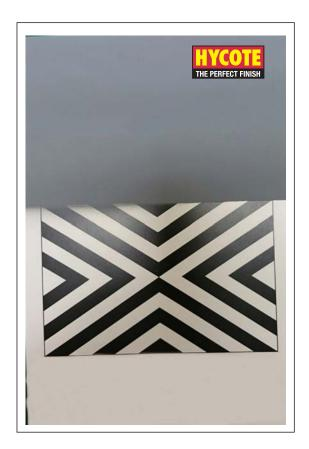
A single coat of paint is applied to contrast cards and allowed to dry in a vertical position. The paint film is assessed for sag resistance and coverage. These images demonstrate superior coverage, sag and run resistance of Hycote primer compared with leading brand C.
