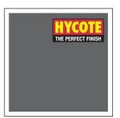
Multiple coats of paint are applied to a contrast card until full coverage is obtained. The card is then dried and the surface appearance and smoothness accessed.
