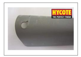
The paint film is bent to an extreme angle in a conical mandrel. Any cracking or peeling of the paint demonstrates poor flexibility. These images demonstrate the superior flexibility of Hycote primer compared with leading brand B.
