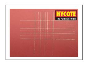
The paint film is cut in a cross pattern before pressure sensitive tape is applied. The tape is removed rapidly to assess adhesion of the paint to the substrate. The more the paint detaches from the surface of the substrate, the worse the level of adhesion. This illustrates the superior adhesion of Hycote red primer compared to leading brand A.
