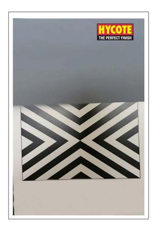
A single coat of paint is applied to contrast cards and allowed to dry in a vertical position. The paint film is assessed for sag resistance and coverage. These images demonstrate superior coverage, sag and run resistance of Hycote primer compared with leading brand C.
